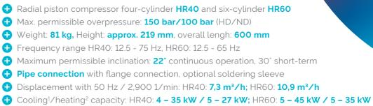
1) based on evaporation temperature +10 °C, superheat 10K, high pressure 100 bar, gas cooler outlet +40 °C 2) related to evaporating temperature -20 °C, superheat 10K, high pressure 80 bar, gas cooler outlet +25 °C
